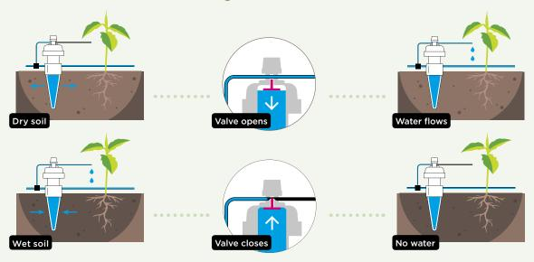
**This is how it works:** the Tropf-Blumat is filled with water. This water is not used for watering but for control. If the soil gets dry, the Tropf-Blumat releases a bit of water onto the soil. The pressure goes down inside as a result and a valve opens. Once the soil is moist enough, the water is drawn back into the Tropf-Blumat through the clay cone and the valve closes. A simple principle of physics but highly effective and reliably for many years.
