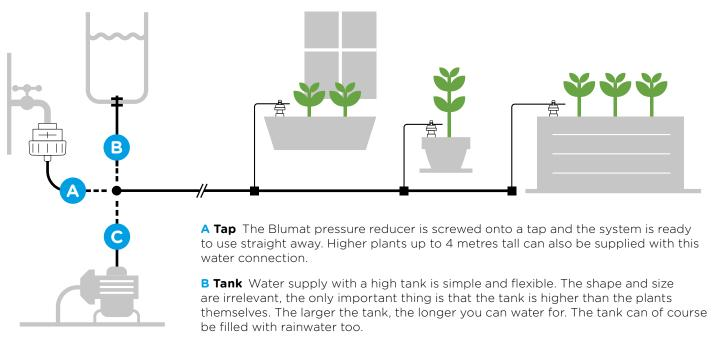
**C Pump** With a pump you can draw in water from a fountain or lower lying tank to supply your Tropf-Blumat system. Only use pumps with an integrated expansion tank (domestic water system) and install the Blumat pressure reducer at the pump outflow. Higher plants up to 4 metres tall can also be supplied with this water connection.
